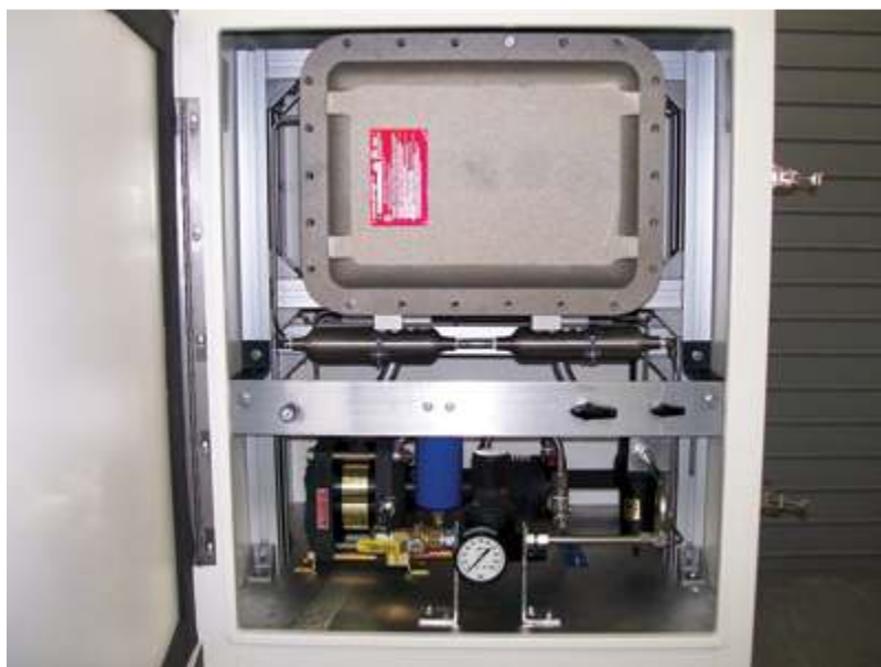
2. Tracking down contaminants. The PlantGard high-pressure gas pipeline contaminant monitor can detect and measure aerosols and solid particles. Data from the monitoring system are normally communicated by serial or analog cable to plant digital control systems. Source: PECOFacet/Scientific Process Solutions Inc.
