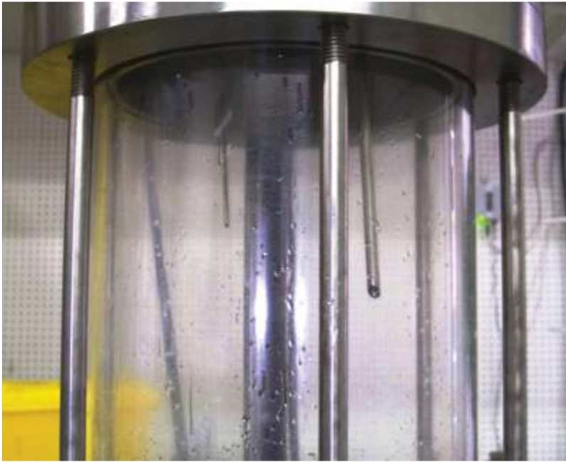
5. Caught in the act. The wet gas flow in the pipeline illustrates a liquid contaminant upset. Source: PECOFacet/Scientific Process Solutions Inc.
